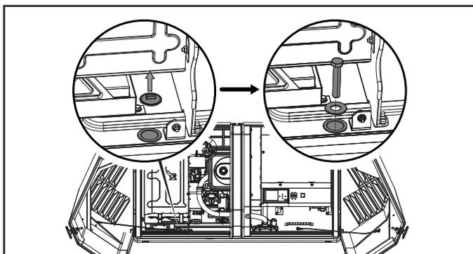
2. Open right door, access hurricane bushing near front alternator side as shown. Remove bushing cap, and install washer and bolt as shown. Bolt and washer will tighten inside the hurricane bushing below the home standby pan. Torque to 3.2 Nm (2.4 lbf-ft) or hand tight and 1/8 turn more.
