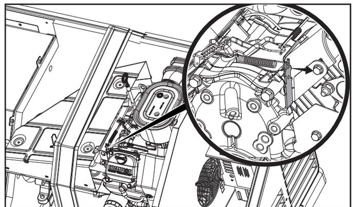
ii. To decrease engine speed HSNL bend the spring anchor tang on the fixed speed controls toward the governor lever to decrease spring tension.
