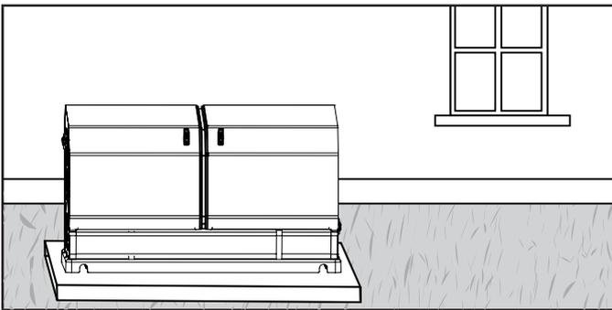
Compact the fill, this is to provide a firm base for the HSB. Remember the final stone level must be 2 or 3 inches (5.1 or 7.6 cm) higher than the original ground level to ensure water run-off and drainage.
