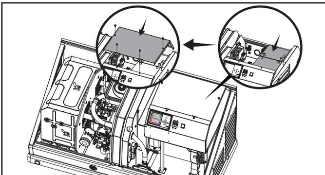
7. Inspect, clean or re-grease battery connections every two months.
