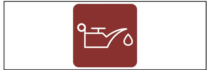
The RED icon will be lit when the engine oil pressure drops below a safe operating level. When this fault is detected, the HSB will shut down and re-start will be disabled. RED icon on the controller module and exterior LED will be lit.
