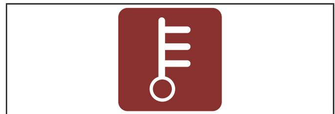
The RED icon will be lit if the engine operating temperature exceeds the factory preset limits. If excessive operating temperature is detected, the HSB will shut down and re-start will be disabled. The RED icon on the aXis Controller® and exterior enclosure LED will be lit.
