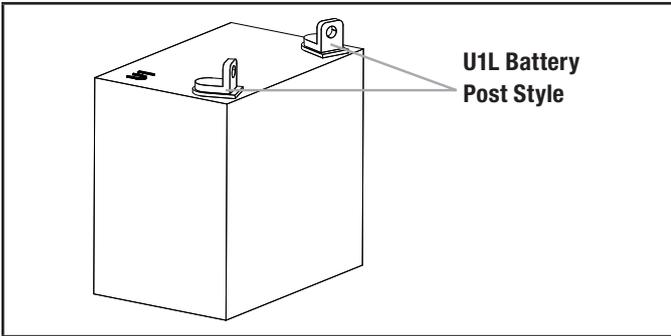
1. Place the batteries in the front right corner of the HSB enclosure. Features on the floor of the enclosure locate batteries. If replacing existing batteries, disconnect wiring and remove old batteries.
