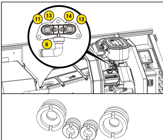
5. Install fuel inlet chamber to mixer body. Tighten fuel inlet chamber screws (3). Screw Tightening Torque: 26.0 lb.-in. (2.94Nm).
