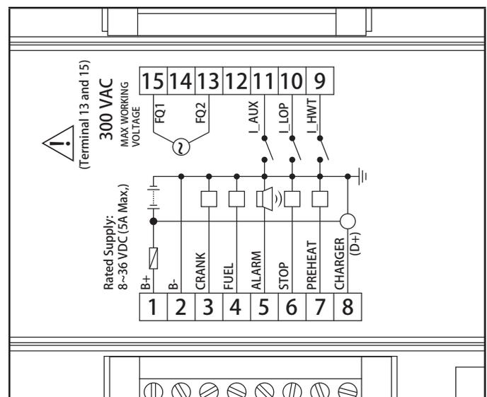
The pins relate to a function of the aXis Controller®. These functions control the operation of the HSB aXis Controller® module. There are 15 pin locations. Remember the icons on the front side of the module are only indicators of a run (GREEN) or fault (Red). These are the designated pin locations, function and wire colors for reference;
