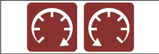
The RED icon will be lit if the engine was operating above or below its preset speed limits. These limits are factory set to protect the HSB and the circuits connected to the generator output circuits. When this fault occurs, the HSB will shut down, light the RED icon, shut down and re-start will be disabled. The exterior warning LED on the back of the HSB enclosure will be activated and lit.
