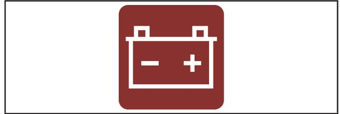
The RED icon will be lit if the battery voltage falls below 21.0 volts for at least 5 seconds while the engine is running. If the battery voltage rises above 22 volts, the icon will turn off. Battery voltage is NOT monitored when the engine is cranking, just when the engine is running. If the RED icon comes on it will not shut the HSB off, it will remain lit until the battery condition meets the required output.
