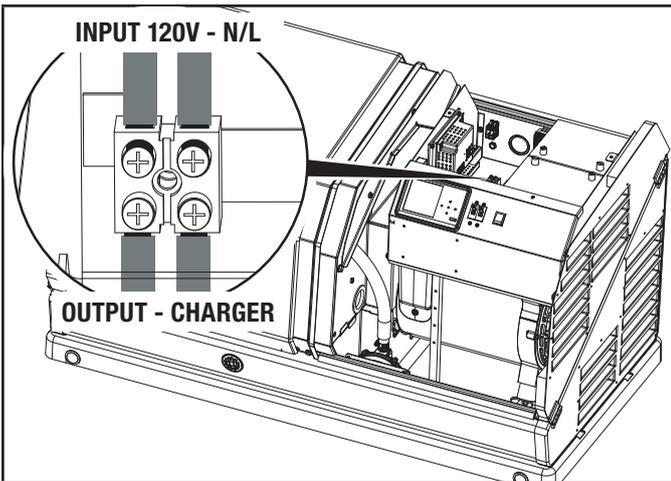
The terminal block is prewired by the factory to the charger L1 and N. A 120 VAC circuit must be installed for battery charging from the ATS or another 120VAC circuit.
