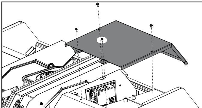
Swing the aXis Controller® panel forward after removing the top cover, HSB starting will be disabled.
