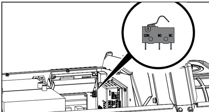
To access this microswitch, remove four M6 x 12 bolts from the cover using a 10mm wrench (not included).
