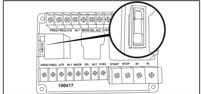
2. An automotive style fuse, 40A (Orange), which protects the system from an excessive transfer voltage output when the ATS relays transfer between utility and generator and generator to utility modes. Remove plastic FUSE cover to access.
