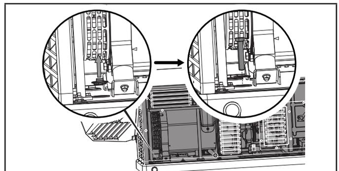
4. From the back side, through the access panel, access hurricane bushing near back muffler side as shown. Remove bushing cap, and install washer and bolt as shown. Bolt and washer will tighten inside the hurricane bushing below the home standby pan. Torque to 3.2 Nm (2.4 lbf-ft) or hand tight and 1/8 turn more.
