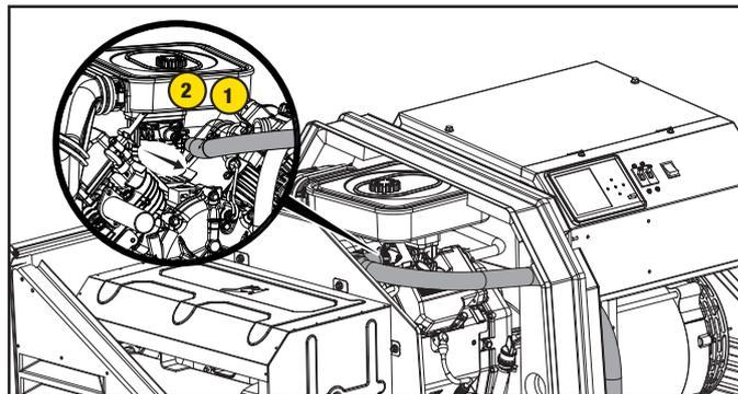
2. Remove P clamp by removing M10 bolt. This will give you easier access to remove and install the Master Mixer Assembly.
