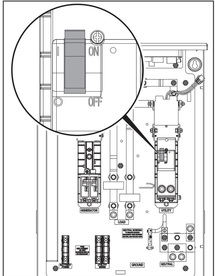
3. With an AC voltmeter, check for the correct voltage. Single-phase utility power supply. Measure across the UTILITY SUPPLY ATS terminal lugs L1 and L2. Also check L1 to NEUTRAL and L2 to NEUTRAL.
