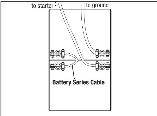
4. Dielectric grease should be applied on the battery connections to aid in the prevention of corrosion.
