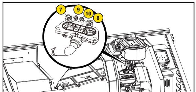
4. Install LPG jets and gasket (6) to fuel inlet chamber.
