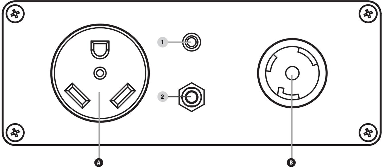
1. **Power Indicator** – Illuminates green when power is being supplied to the parallel kit.
