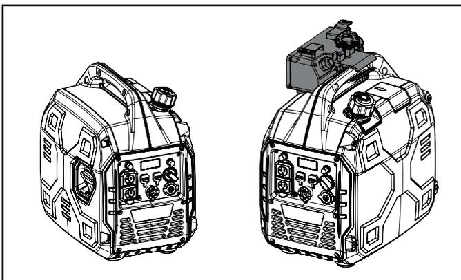
4. Place the bracket around the handle and tighten the fastening dial by turning clockwise until snug. Do not over tighten. You may need to loosen the fastening dial to get it around the handle before tightening.
