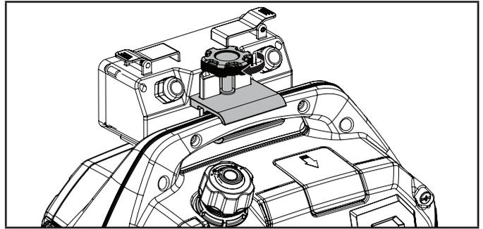
5. On each inverter, lift the parallel port covers, if applicable, and insert the RED power lead into the RED receptacle and the BLACK power lead into the BLACK receptacle.
